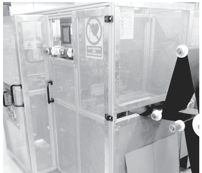
Photo 4. High frequency welder No. 1: a) before the shielding installation, b) after the shielding installation
